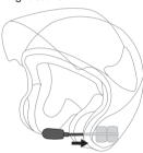
Note: HOLA headset provides quality voice and VOX intercom. For optimal performance, the microphone must be as close to the mouth of the user as possible when installing the microphone.
