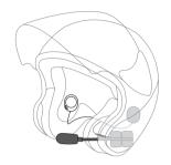
Step 3: Pull to open the clip of the HOLA headset fixture and clip/slide onto the lower rim of the helmet. To further enhance the fastening, remove the adhesive protection paper from the back of HOLA headset fixture before fastening the headset fixture to the helmet. Caution:
